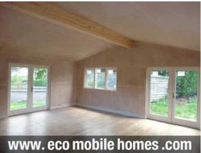
**Internal Carpentry.** Standard finish is real wood oak flooring and doors with painted MDF skirt, all in a choice of styles. Extensive range of alternative finishes available.
